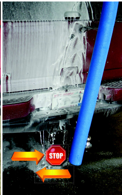
Sensing deflection, motion stops, automatically reverses direction...
